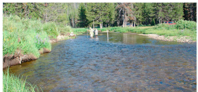
Figure 2. Field conditions. Measuring discharge in upper Bear Valley Creek at an intermediate flow stage. View is downstream.
