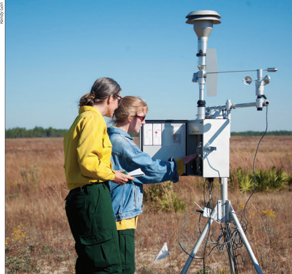
Station scientists check an instrument for measuring smoke concentrations downwind from a research burn conducted at Eglin Air Force Base, Florida.
