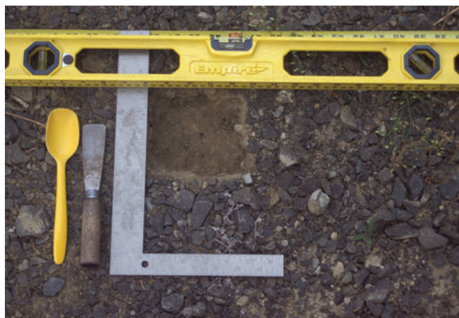
Fig. 3. Excavation of 0.2 m × 0.2 m hole for the large portion of a nested aggregate sample. The square indicates the 0.1 m × 0.1 m hole for the small portion referred to in Fig. 2.
