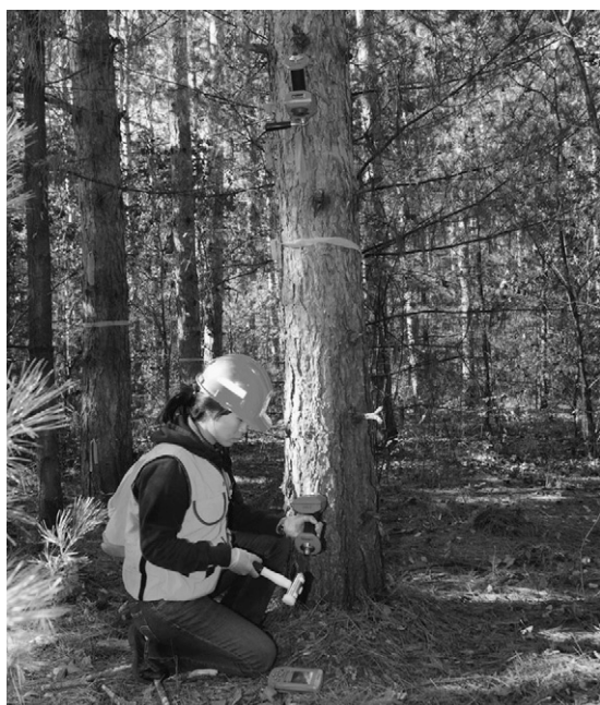
Figure 1. Field acoustic measurement on standing red pine ( Pinus resinosa ) trees.
