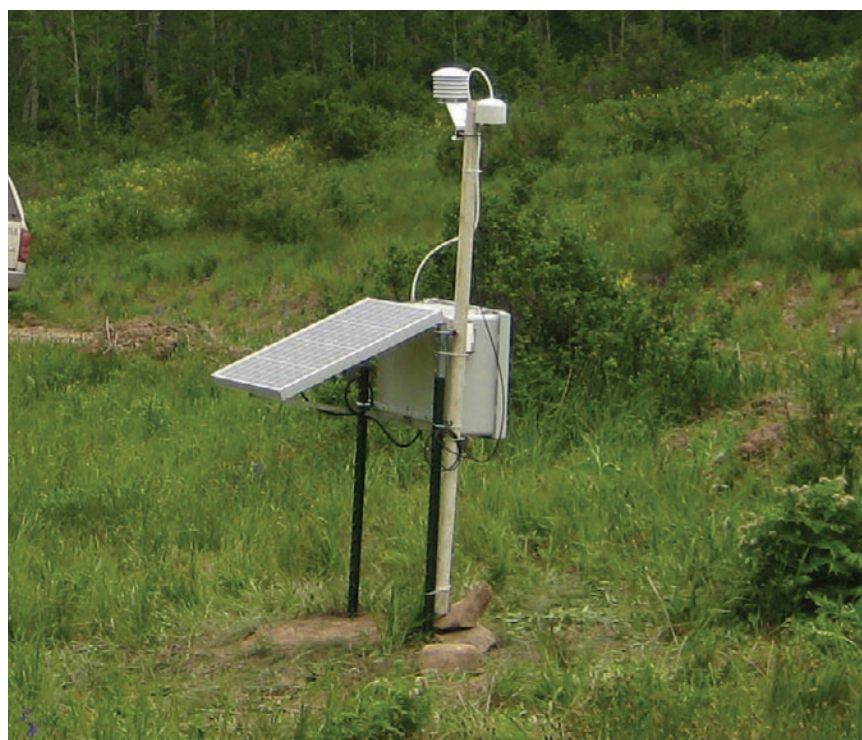
Figure 4 —Version 5.0 installation showing 40W solar panel, instrument/battery enclosure, and sample inlet support (Gunnison National Forest near McClure Pass, Colorado).
