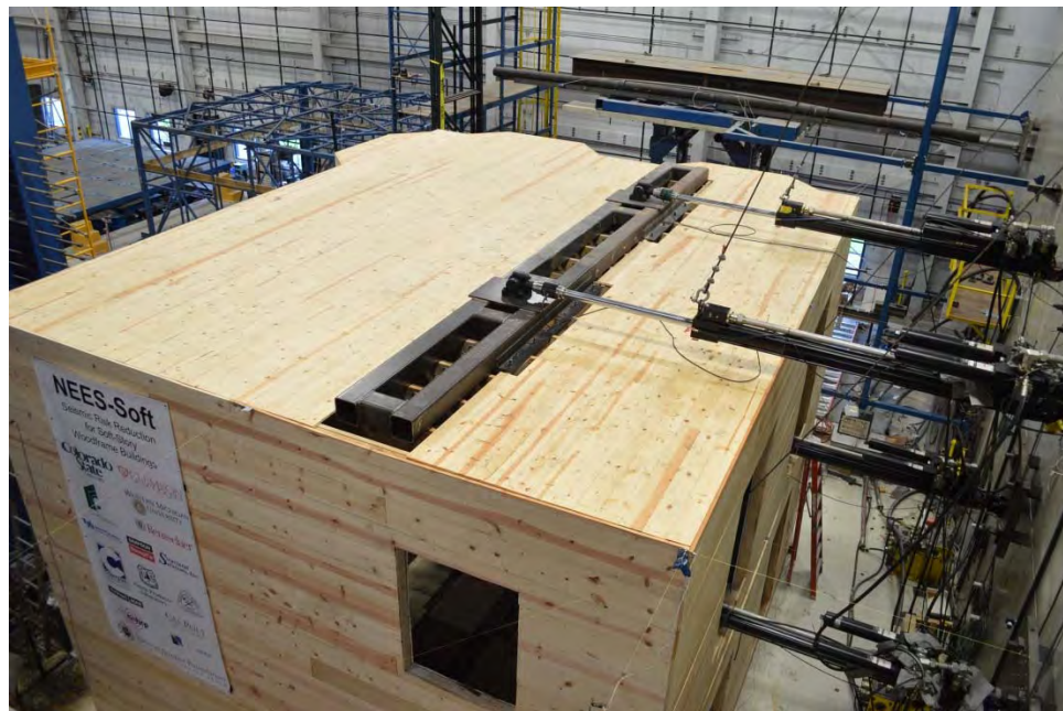
Figure 3. The hybrid test building at the NEES@Buffalo laboratory
