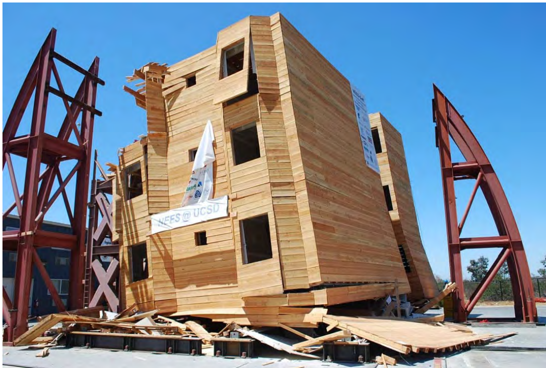
Figure 11. The collapsed NEES-Soft test building on the shake table at NEES@UCSD.
