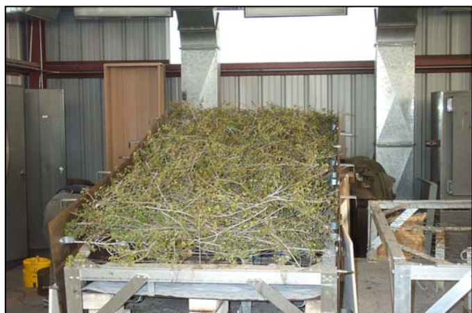
Figure 3. Experimental fuel bed constructed of Ceanothus crassifolius branches and foliage < 0.6 cm. Fuel bed density is greater than normal density and fuel bed is elevated 40 cm above surface.
