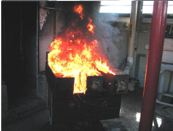
Figure 1: Flames in wood crib of creosote-treated timbers ~30 s after application of hot metal wafer
