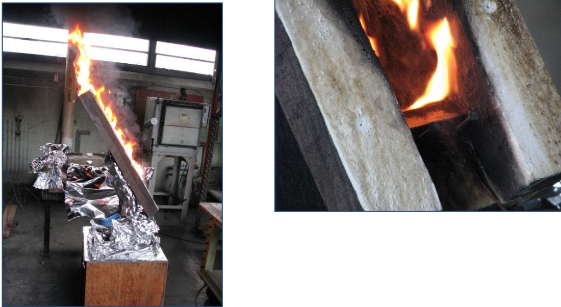
Figure 3: Hot metal test apparatus (left) and ignition source (right)
