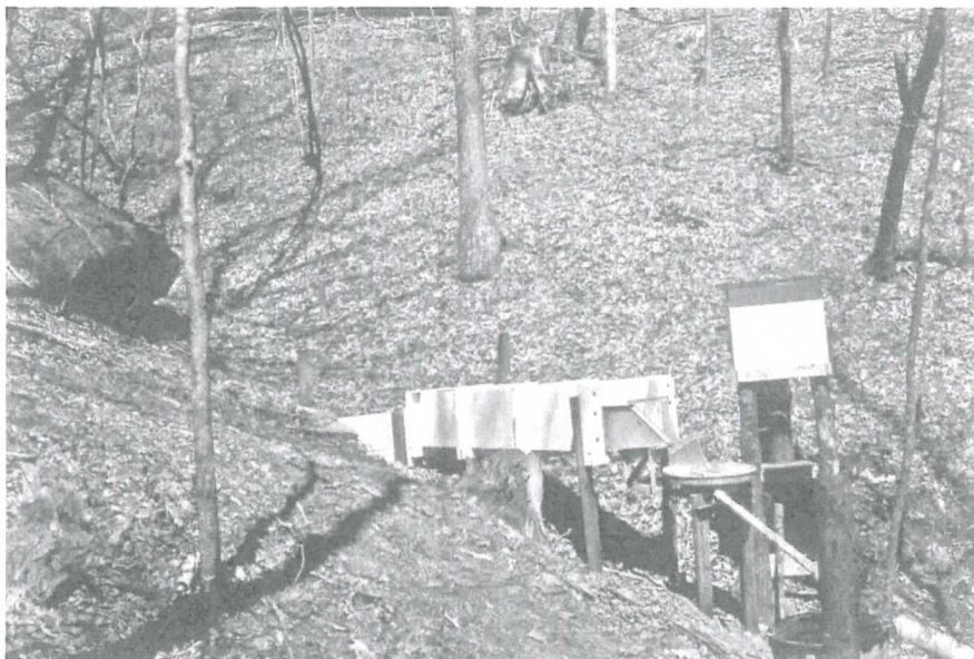
Figure 3.9 One foot H-Flume and Coshocton sampler (no. 701) on WS 7—one of four such installations used to assess water quality above and below roads, 1976. (USDA Forest Service photo)
