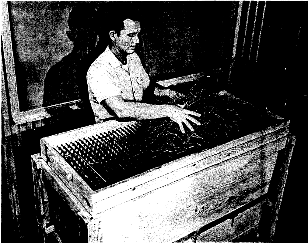
Figure 2. --One pound of loblolly pine needles is placed on the top of the fabricator. After the needles are uniformly distributed over the grate, they will be moved into position between the bars and allowed to free fall into the tray below.
