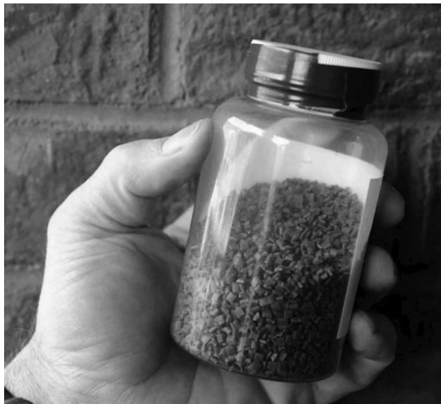
Figure 4. Biodegradable flakes ( \sim 3 \text{ mm}^2 ) containing verbenone suitable for aerial applications.
