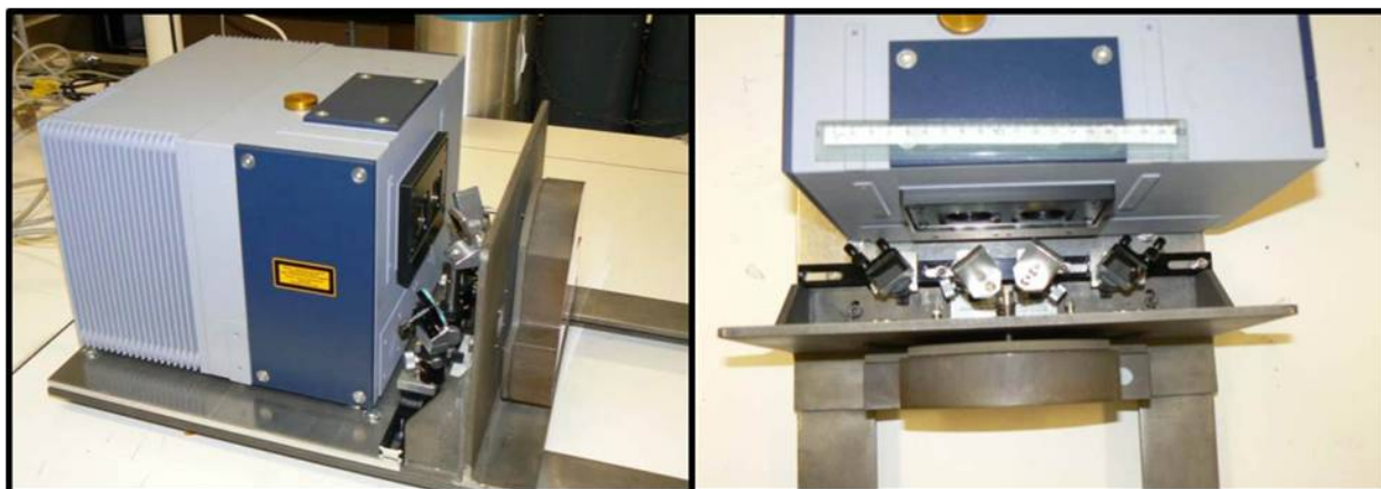
Figure 3.2 FTIR, transfer optics, cell entrance and field mirror. Most of cell is not seen in the photograph. The cell spans the stack \sim 15 m above the fires at the Fire Science Lab as seen in the cartoon of Figure 3.1
