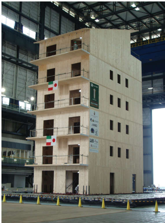
Figure 10 Seven-story CLT house tested at E-Defense Laboratory in Miki, Japan
