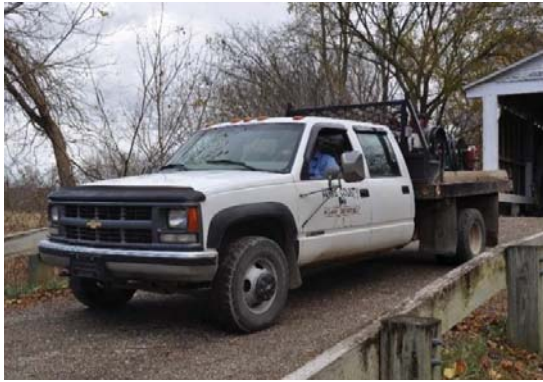
Fig. 3 Small truck used for load testing the Cox Ford Bridge
