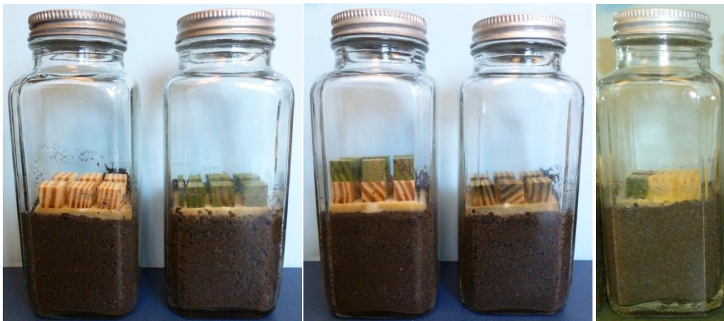
Figure 2.3 Variations on copper citrate (CC) – treated test blocks exposed to F. radiculosa . Bottle 1: untreated SYP; Bottle 2: CC treated SYP; Bottle 3: CC treated SYP on top of untreated SYP; Bottle 4: liquid CC on top of untreated SYP; Bottle 5: CC treated SYP adjacent to and in direct contact with untreated SYP.
