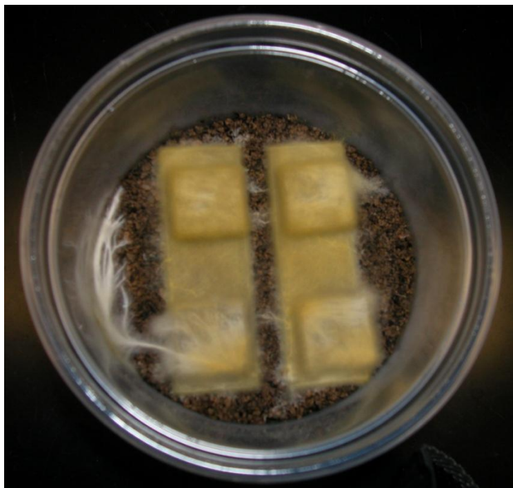
Figure 2.1 Decay chamber set-up including feeder strips and test wafers exposed to isolate, L-11659-SP.
