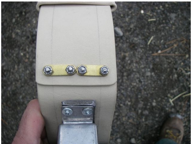
Figure 3. Two-piece expandable Kydex collar, which shows the attachment with 2 standard belt-collar stud-plate-nut closures. This design allowed us to fit collars on mature male elk.
