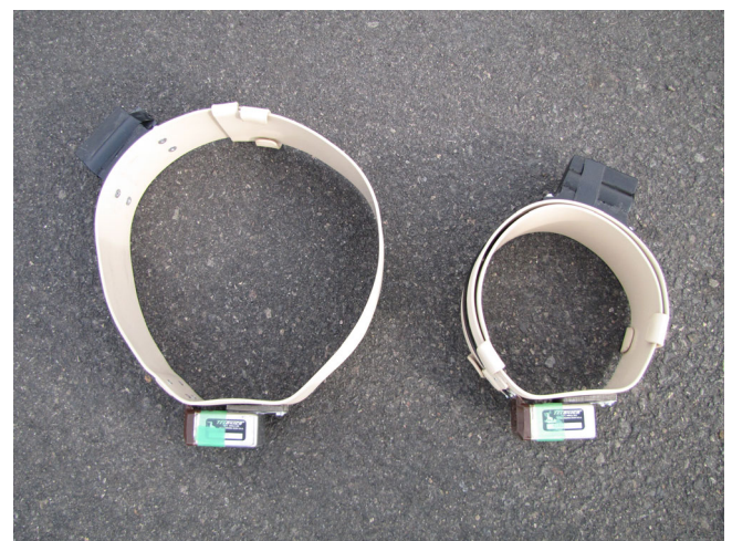
Figure 2. Self-adjusting expandable collar with very high frequency transmitter and global positioning system unit attached. Maximum circumference (left) was 90 cm, and minimum circumference (right) was 60 cm.
