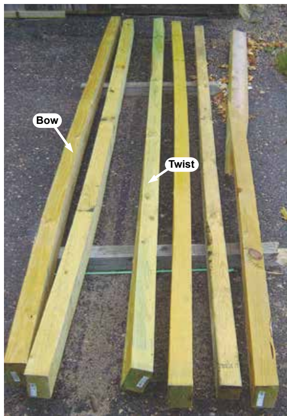
Figure 23. Examples of bow and twist in sign posts. Source: Matt Rauch, WisDOT.
