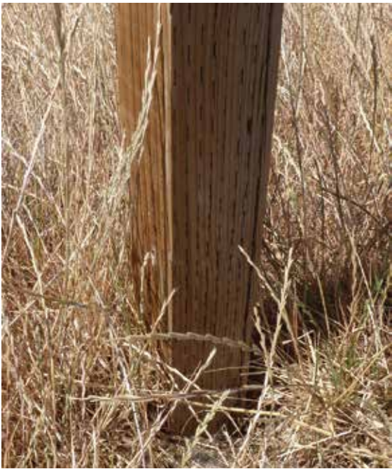
Figure 12. Incising is used on less treatable wood species to improve depth and uniformity of treatment.
