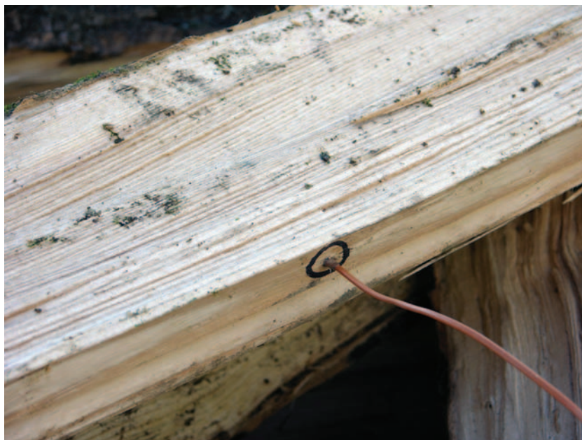
Figure 2. Thermocouple wires were inserted into the center of firewood samples at the midsection.
