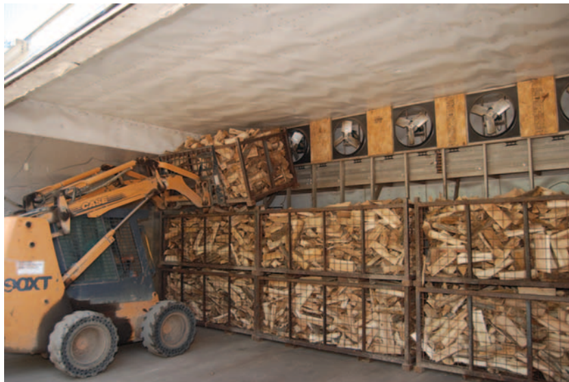
Figure 1. Firewood baskets are placed into the kiln. The monitoring firewood samples were placed in the three baskets of the back row in the lower level. One instrumented piece was placed into each basket.
