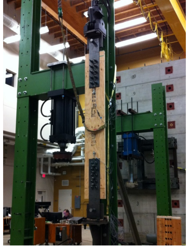
Figure 3: Multiple bolted connection test setup
