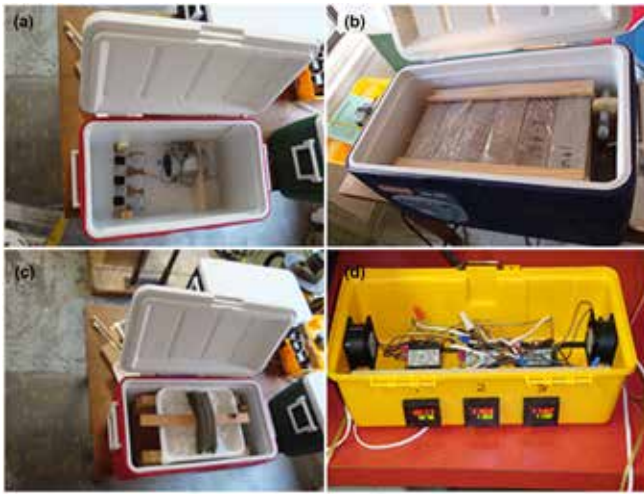
Figure 2. Conditioning chambers showing incandescent bulbs and fan assemble (a), loaded with samples, with yellow thermometer protruding from a hole in the left side and a data logger on the right side (b), with salt pan installed and with foam spacer to divert air flow (c), and control box showing three control assemblies with temperature read-outs visible in front (d).
