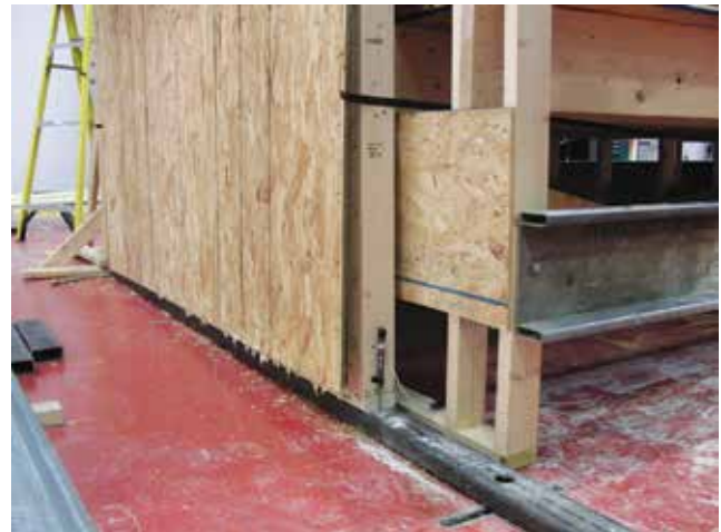
Figure 13. Fastener pull-through failure mode of Test C and Test D.
