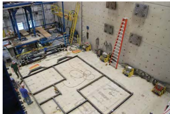
Figure 3. Steel interface plate and strong wall at NEES@Buffalo
