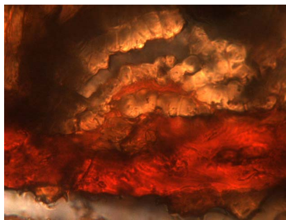
Figure 3. Light microscopy image (40X cross section) showing a red phenol-resorcinol-formaldehyde adhesive flowing into tannish libriform separated cells of lpe.
