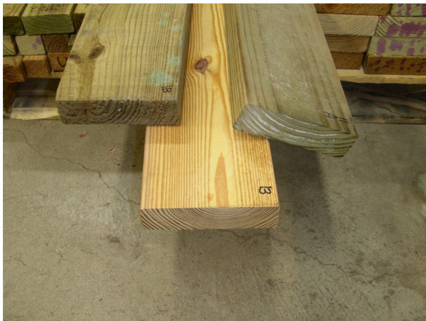
Figure 3. (From left to right) Wood treated with MCQ, DDAC, and ACQ. Cupric ions from the wood preservative cause the dark coloration of the wood. Excess copper has deposited on the MCQ (green splotches) and the ACQ (along the end grain) samples. SCALE: The boards are approximately 38 × 140 mm.
