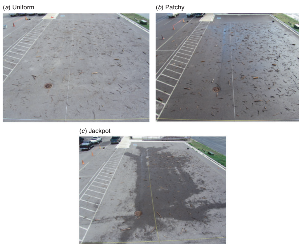
Fig. 1. Layout of fine woody debris (FWD) surface fuelbeds in the parking lot of the Missoula Fire Sciences Laboratory for the three fuel distributions: (a) uniform – even distribution of FWD across the 500-m 2 plot, (b) patchy – 80% of FWD is evenly distributed in half the plot and (c) jackpot – 50% of fuel is evenly distributed in a quarter of the plot and the remaining 50% is evenly distributed across the other 75% of the plot.
