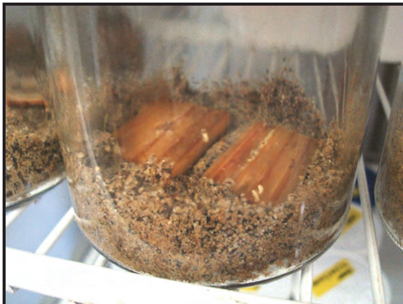
Figure 1: Choice test jars with two wood specimens and termites
