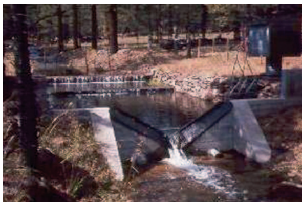
Fig. 14.1 Castle Creek East Fork was monitored with 120-degree v-notch weir. The objective on the two Castle Creek watersheds was to start management of the ponderosa pine forest to a system using a 120-year rotation with 20-year cutting cycles. East Fork was the original control watershed but a preharvest watershed prescribed fire treatment was evaluated after 1981. (Photo by G. Gottfried)
