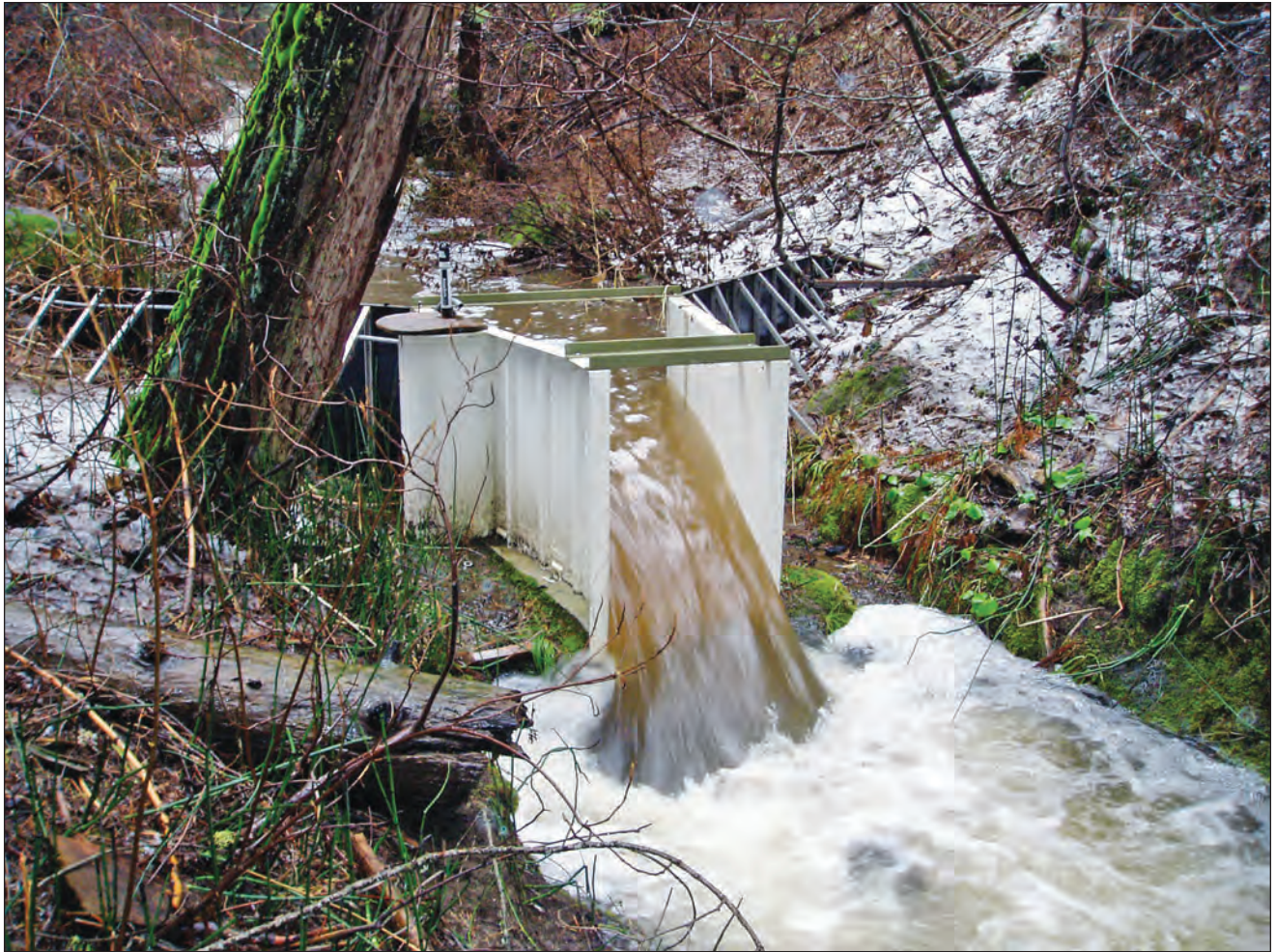
Figure 5—Intense rain events or rain-on-snow events can increase suspended sediment and turbidity in streams, as shown at one of the flumes in the Kings River Experimental Watersheds, Sierra National Forest.
