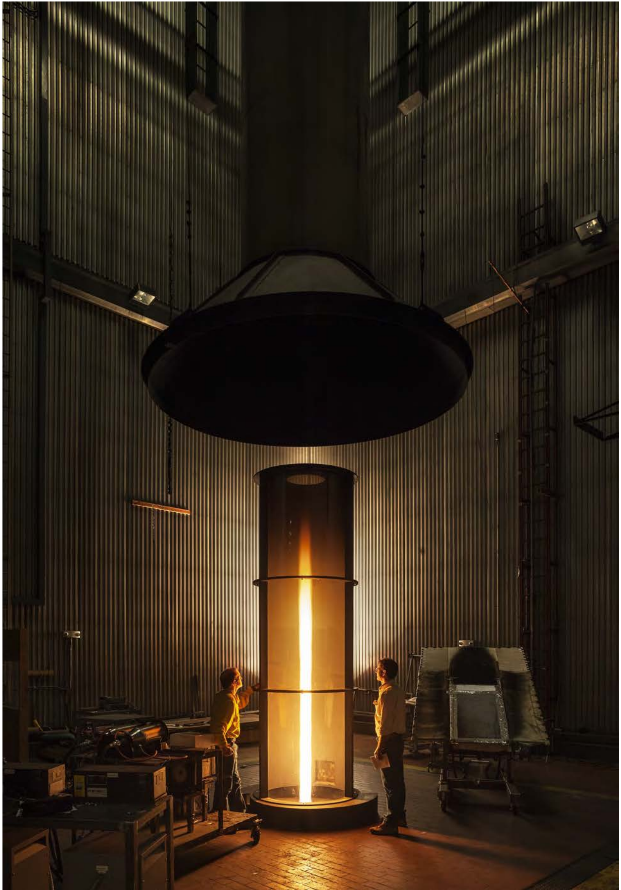
Photo: Burn chamber at the Missoula Fire Sciences Laboratory, showing the fire whirl generator. The burn chamber is 40 feet wide, 40 feet long, and 70 feet tall. Made of metal and concrete, it provides a climate-controlled laboratory for research. Photo courtesy of Richard Barnes / OTTO.
