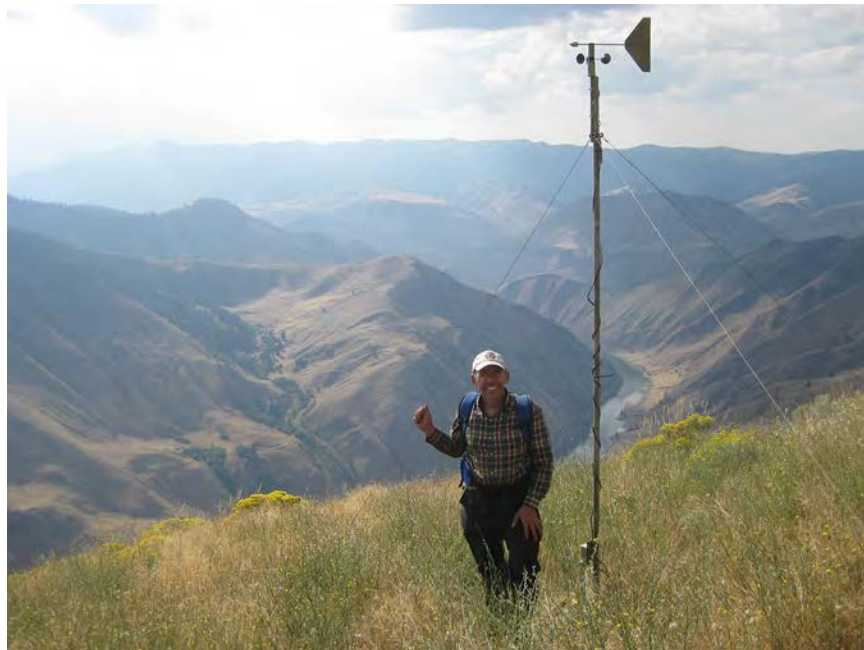
Photo: FFS Physical Scientist Mark Vosburgh stands next to a wind anemometer installed to improve the accuracy of models used to simulate wind speed and direction in complex terrain.
