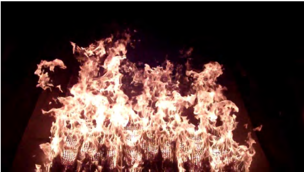
Photo: Downwind view of fire spreading through laser-cut cardboard fuel beds in the Missoula Fire Sciences Laboratory's wind tunnel. The U-shaped depressions from left to right are related to the presence of Görtler vortices that force the fire downward into the fuel bed.
