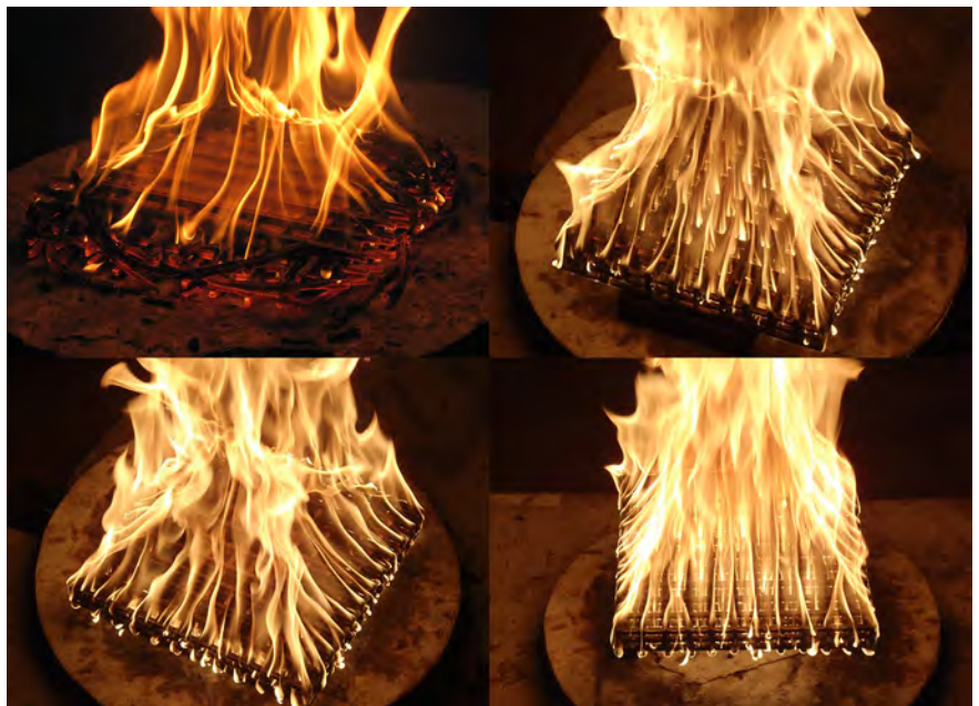
Photo: Change in burning regime for a large length-to-thickness ratio crib as the crib-platform spacing increases. Clockwise from top left: no spacing; 1.27 cm (0.5 in) spacing; 7.62 cm (3 in) spacing; and 2.54 cm (1 in) spacing. Photos courtesy of Sara McAllister / FFS.
