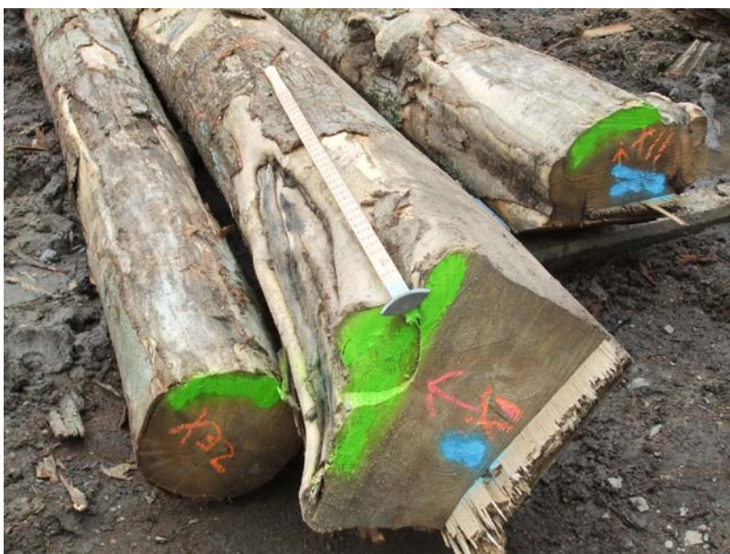
Figure 1.—Red maple logs from Fernow Experimental Forest, West Virginia, at sawmill log yard with paint and arrows designating the face on each log that was affected by fires and a log identifier (X32, X1, X11) for use in tracking the lumber sawn from each study log.
