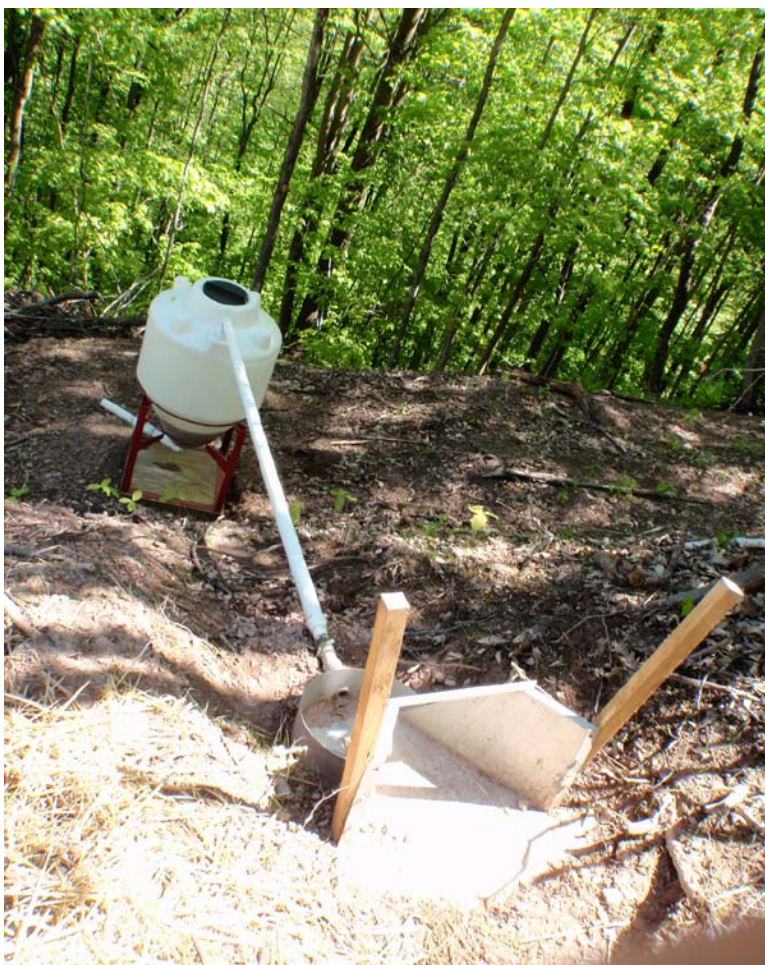
Figure 2.—Photograph showing a sediment collection device at a waterbar outlet. Runoff and sediment collected in the flume were diverted downslope into a collection tank by gravity. Samples were collected from a spigot at the base of the tank. Photo by Pam Edwards, U.S. Forest Service.
