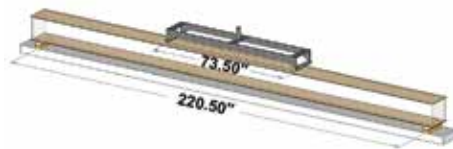
Figure 2. FPL static loading diagram.
