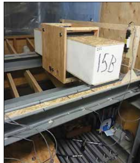
Figure 7. Creep test setup (APA-The Engineered Wood Association).
