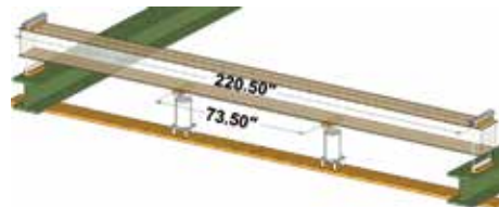
Figure 3. Creep loading diagram (FPL).
