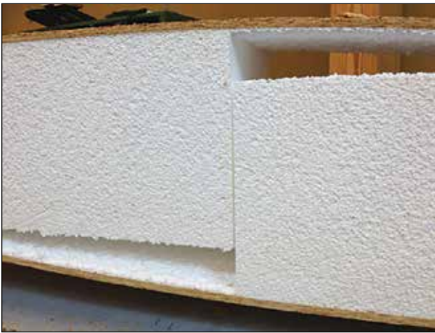
Figure 12. Adhesion failure (FPL).
