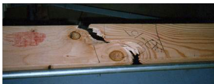
Figure 3. Failure under loading often occurs where edge knots or grain deviation around knots is present.
