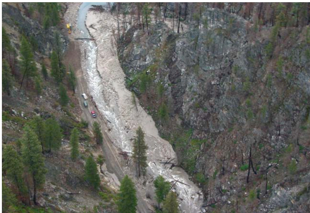
Massive erosion following the Hot Creek Fire near Atlanta, ID, in 2003 caused damage to roadways and stream ecosystems along the Boise River. The fire burned about 27,000 acres and took three weeks to contain. Photo by Charlie Luce.
