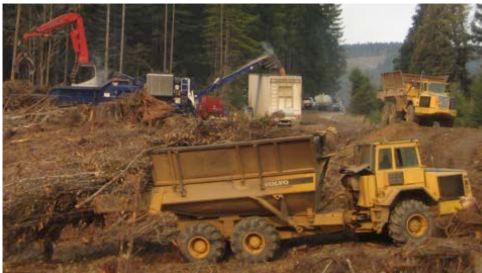
A modified dump truck equipped with higher sides (to allow it to transport forest residue) and skidder tires (for improved forest accessibility). (Image credit: Joel Bisson)
