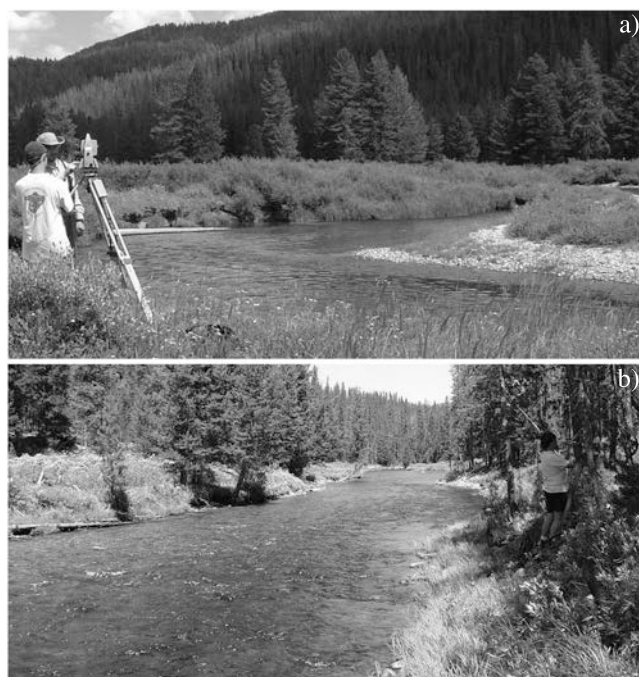
Figure 1. Field sites: (a) Low gradient meandering gravel bed, pool-riffle reach. Channel is approximately 15 m wide. View is downstream. (b) Straight gravel bed channel reach with plane bed morphology. Channel is approximately 15 m wide (see figure on right bank for scale). View is downstream.
