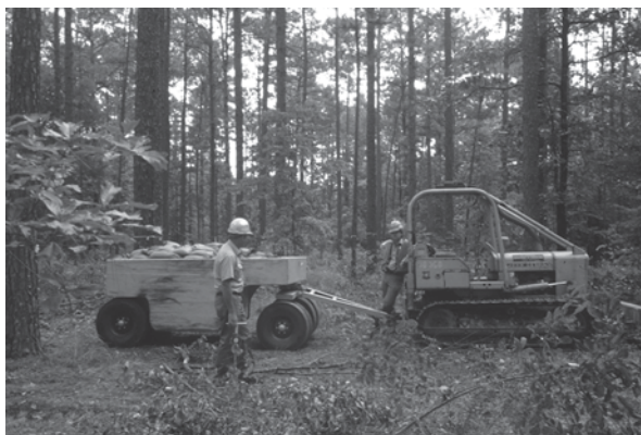
Fig. 23.5 Tractor-drawn Wobble Wheel used in our first soil compaction effort. Note ballast for adjusting the Wobble Wheel load
