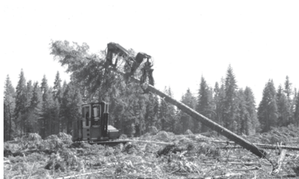
Fig. 23.8 Whole-tree removal was accomplished either by a shovel loader operating from the buffer as shown or by cable suspension. Both methods avoid vehicular traffic on the plots
