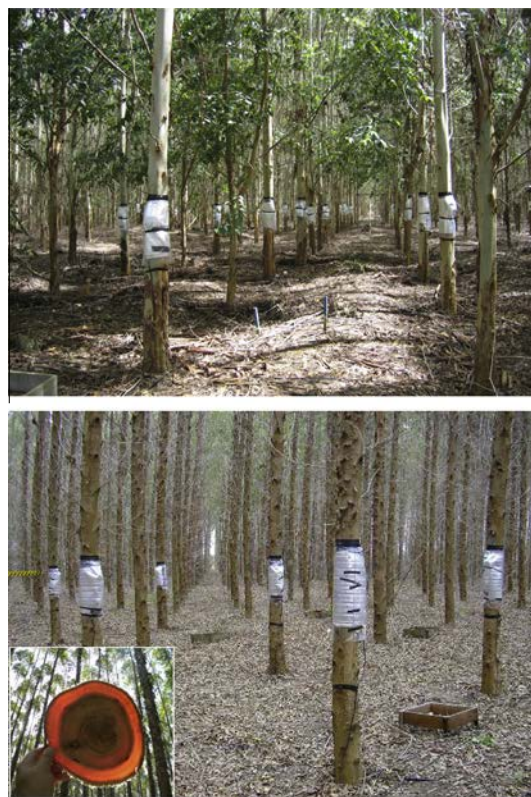
Fig. 1. Instrumented trees at the Aracruz site (upper, clone ARA3918, 38 m 3 ha -1 yr -1 ) and Eunapolis site (lower, clone VER43, 60 m 3 ha -1 yr -1 ) at 5 yr-old in Brazil and visualization of sapwood thickness and area for VER43.
