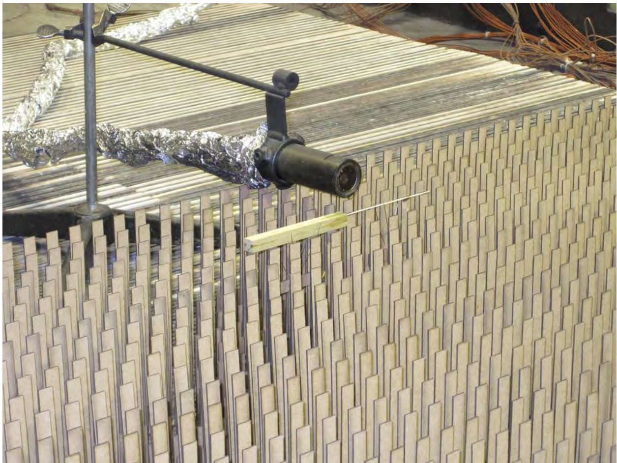
Photo: An instrumented fuel bed composed of laser-cut cardboard. These uniform fuel beds are burned in the wind tunnel to determine rate of spread and other physical characteristics of fire. Photo courtesy of Jack Cohen / FFS.
