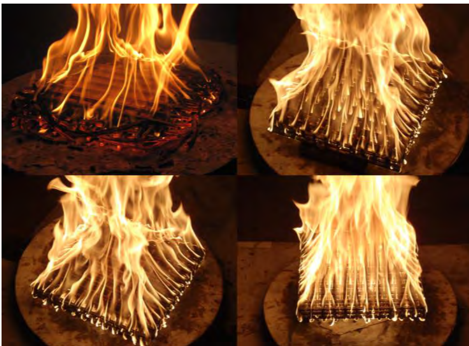
Photo: Change in burning regime for a large length-to-thickness ratio crib as the crib-platform spacing increases. Clockwise from top left: no spacing; 1.27 cm (0.5 in) spacing; 7.62 cm (3 in) spacing; and 2.54 cm (1 in) spacing. Photos by Sara McAllister / FFS.
