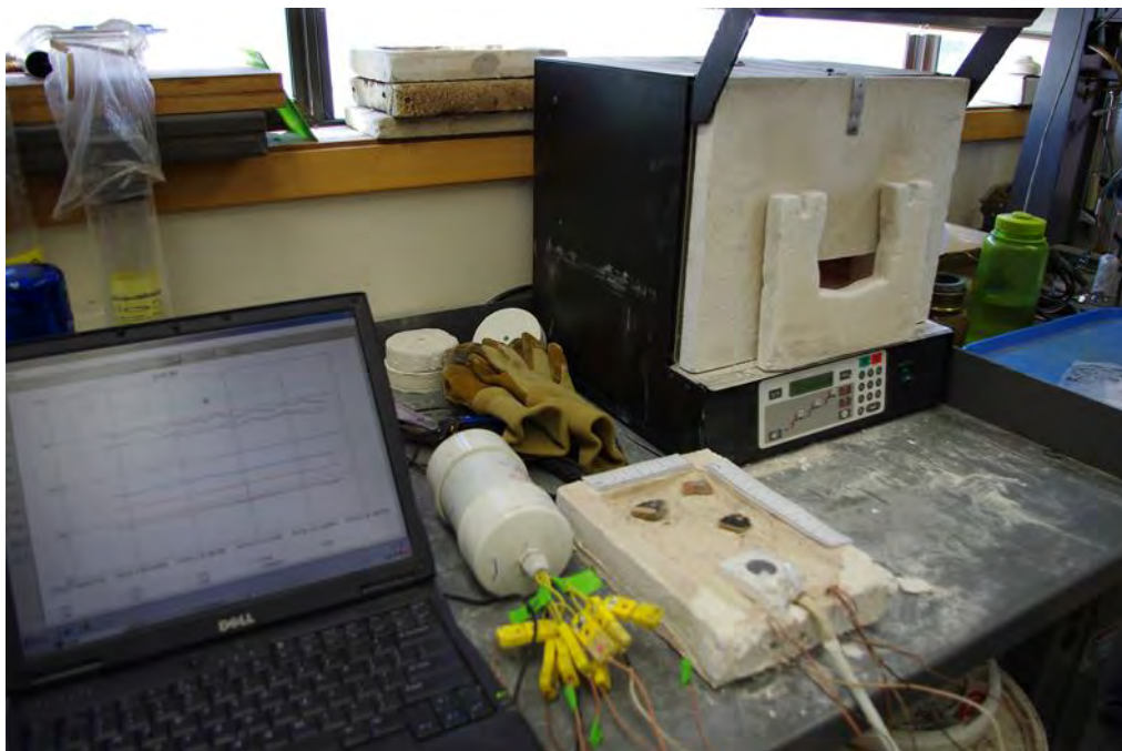
Top photos: Ceramic shards are placed on a bed of sand, instrumented, and exposed to radiant heat in a kiln (left). The ceramic shards are later inspected for damage. The artifacts are exposed to radiant heat of varying temperatures in the kiln (right). Bottom photo: Artifacts were also exposed to heat in a muffle furnace to measure the effects of both radiant and convective heating. Photos by Rebekah Kneifel /FFS.
