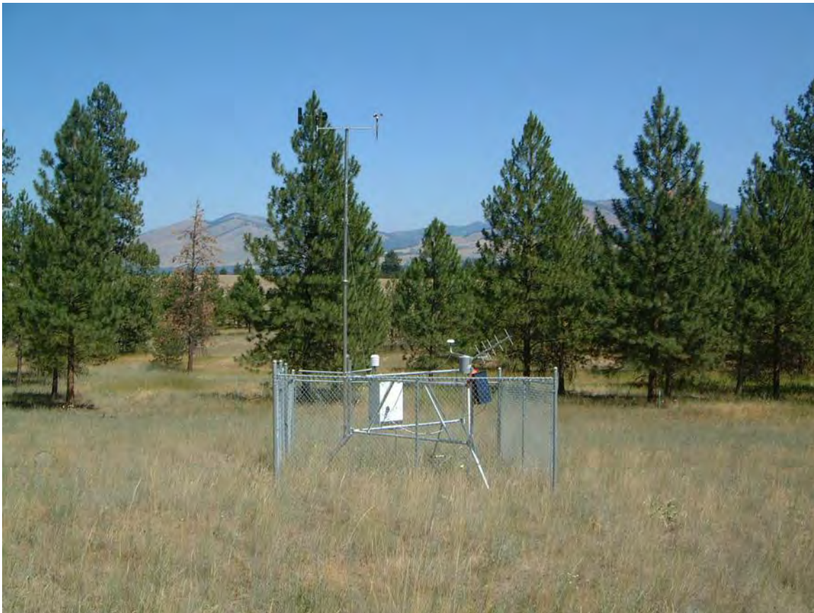
Photo: Remote Automated Weather Stations, such as this one in Missoula, Montana, provide key inputs to the U.S. National Fire Danger Rating System.
