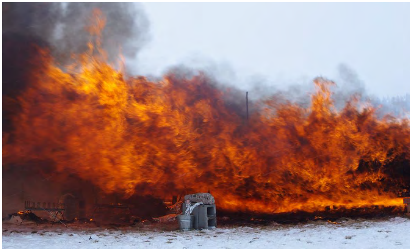
Top photo: Ceramic shards were burned to examine the effects of both prescribed and wildland fire on cultural artifacts. Bottom photo: An outdoor crib burn was conducted in 2014 to examine the effects of heat on architectural stone, shown in the bottom center of the image. Thermocouples were inserted in the stone to measure how heat is transferred through the stone. Afterwards, the stone was inspected for damage. Photos by Rebekah Kneifel / FFS.
