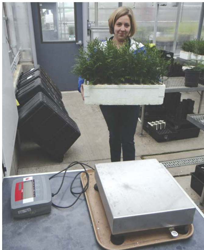
Figure 1. Carrying containers to a stationary balance is one way to determine container weights. This works well where distances are short and only one balance is required. Photo by R Kasten Dumroese
