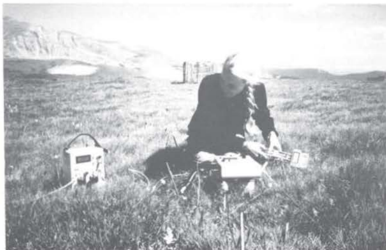
Anna Schoettle measuring gas exchange of alpine plants with a portable photosynthesis system
