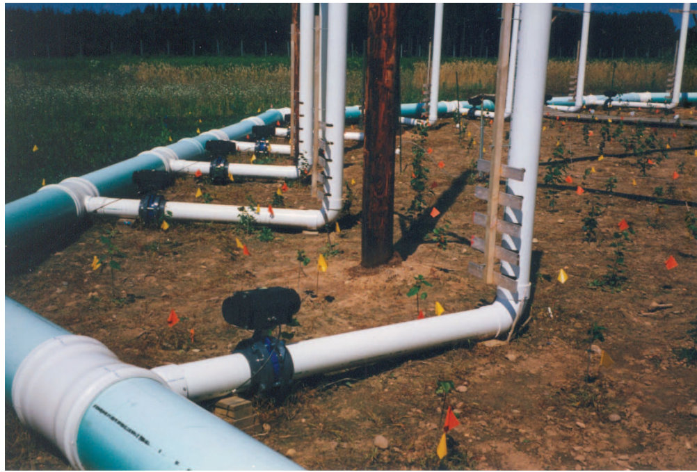
Figure 3.—Portion of a treatment ring showing plenum, vertical vent pipes, aluminum deflectors, and pneumatic butterfly valves. Photo by U.S. Forest Service.
