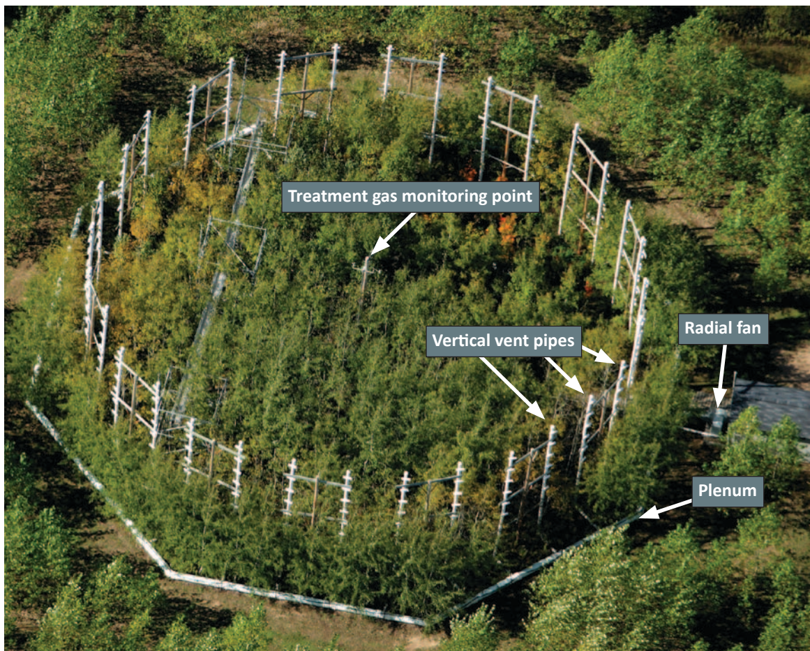
Figure 2.—A typical treatment ring showing the vertical vent pipes, plenum, radial fan, and the location of treatment gas and wind monitoring for control of gas concentration. Photo by D.F. Karnosky, Michigan Tech, used with permission.
