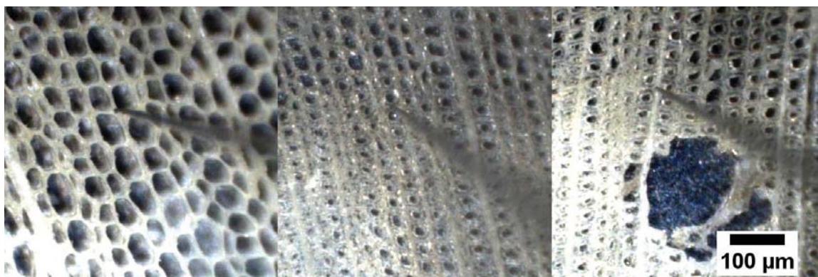
Figure 2: From left to right: example images showing probe placement in earlywood cells, in the S2 layer of latewood cells, and in the middle lamella in the latewood cells.
