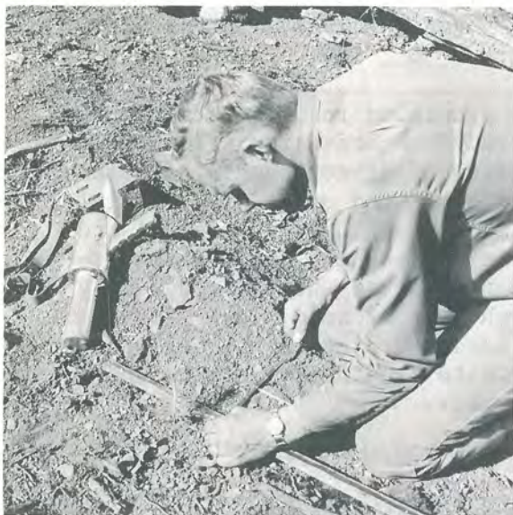
Figure 2.--Radio-tagged seed was located by a sodium-iodide crystal scintillator. Seed is at the tip of the 6-inch plastic marker half way between hands.
