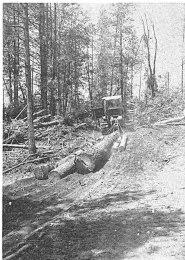
Fig. 2.—Skidding former seed trees to a nearby landing. Nearly 90 percent of all "turns" contain four to five logs. Challenge Experimental Forest, California, December 1963.
