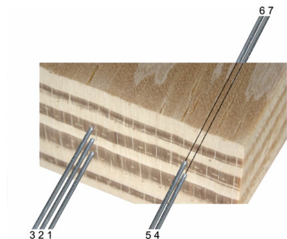
Figure 1. Schematic illustration of the configuration of the electrodes (not to scale). The distance between the electrodes was an experimental variable. The needles were arranged such that every combination of radial/tangential/longitudinal measurement could be taken (see Table I)
