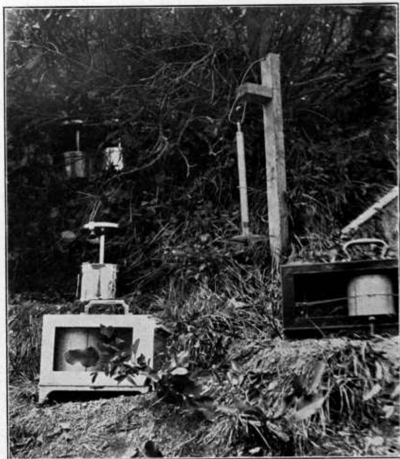
FIGURE 2.—View of instruments as installed for a study of evaporation and temperature in relation to Ceanothus brush
