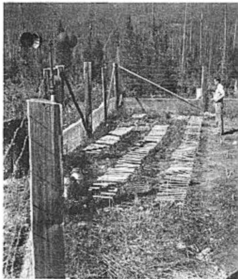
Fig. 1.—The exposure of 230 wood cylinders to eliminate erratic samples and thereby insure comparable measurements.
