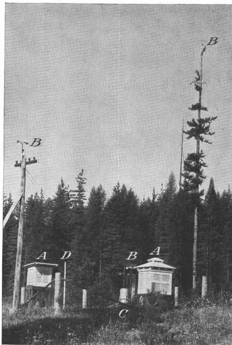
FIGURE 2.—Weather-instrument installation: A , Two types of instrument shelter; B , anemometers exposed at elevations of 9, 20, and 150 feet, respectively, above the ground; C , tipping-bucket rain gage; D , snow stake.
