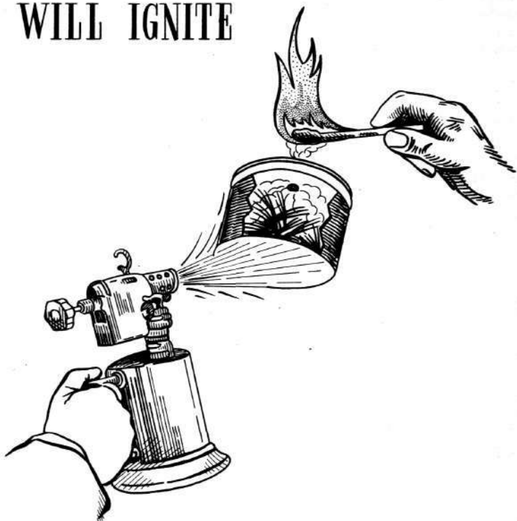
Figure 6. Heat applied to a coffee can full of pine needles will generate ignitable gases. In the combustion process the visible flames are actually burning gases liberated by heated fuel.
