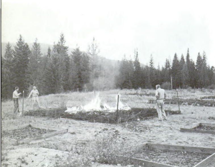
Figure 22. One year's aging considerably reduces peak intensity of fire in slash that loses its needles during the year after cutting (Douglas-fir, 32.5 tons per acre). Upper , current year's slash with needles attached; lower , 1-year-old slash with needles fallen.
