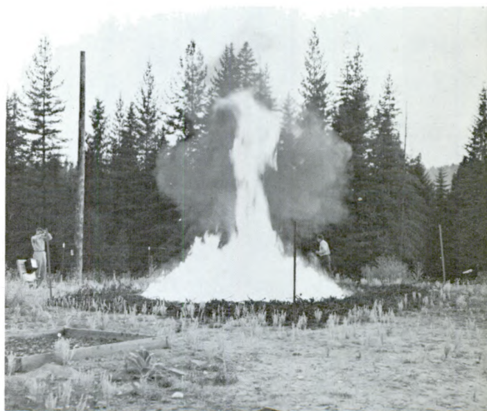
Figure 23. Aging for 1 year only slightly affects peak intensity of fire in slash that retains its needles (western white pine, 32.5 tons per acre). Upper , current year's slash; lower , 1-year-old slash.
